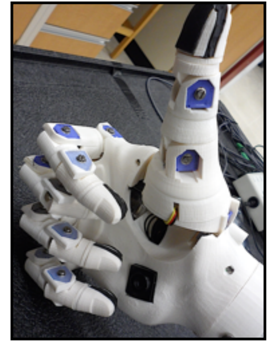
HANDi Hand 6 DoF + 25 Sensors + Camera
