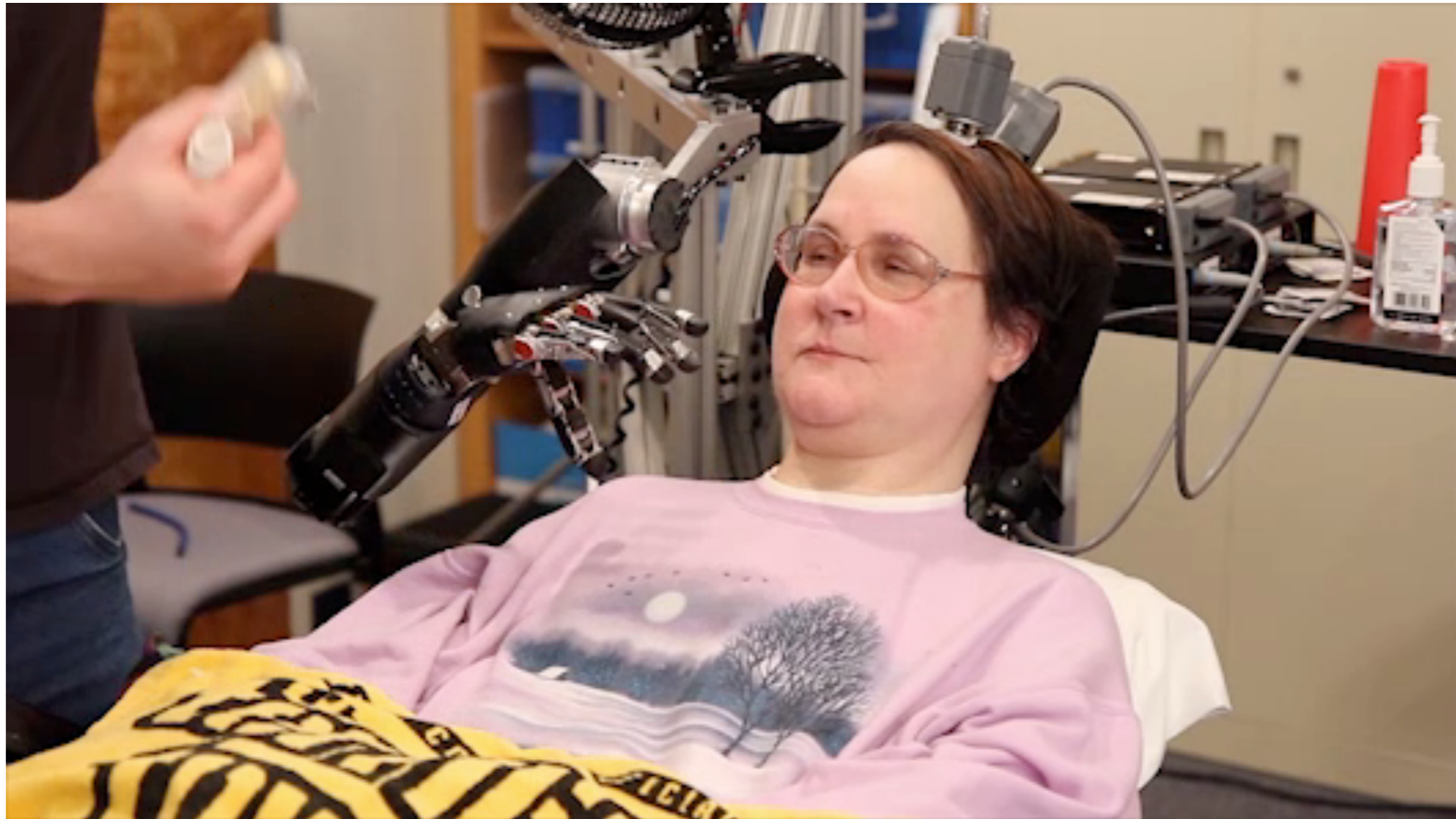
Direct brain-computer interfaces: study participant Jan Scheuermann feeding herself with a robotic limb (University of Pittsburgh) http://www.upmc.com/media/media-kit/bci/Pages/default.aspx
