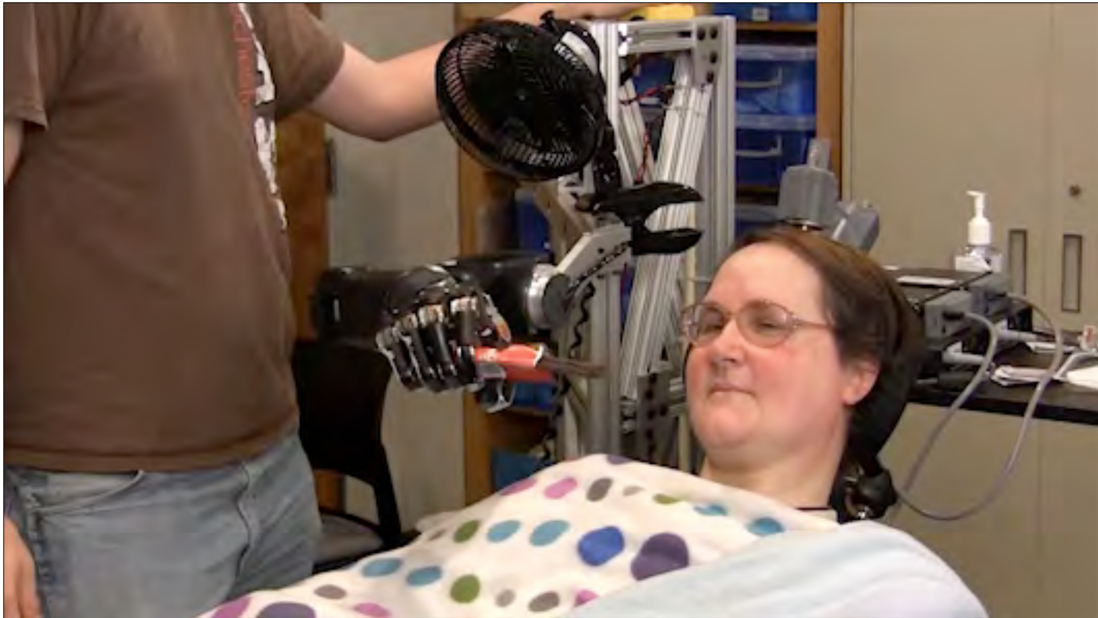
Direct brain-computer interfaces: study participant Jan Scheuermann feeding herself with a robotic limb (University of Pittsburgh); http://www.upmc.com/media/media-kit/bci/Pages/default.aspx
