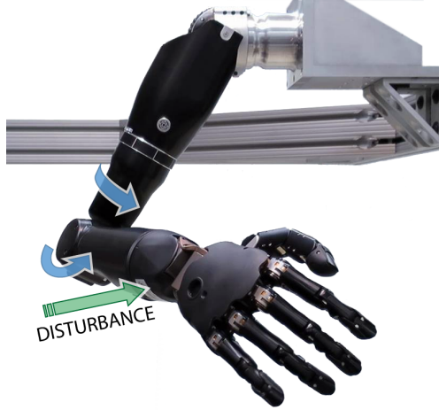
Figure 4.3: The Modular Prosthetic Limb (MPL) used for the experiments. The arrows indicate the nature of the repeated disturbance imposed during the experiment. The green arrow indicates the direction of the provided perturbation, while the blue arrows indicate the resulting joint movement.
