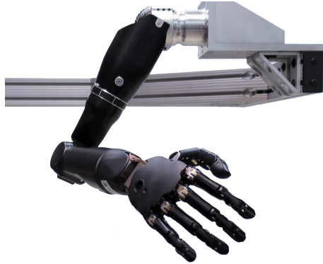
Figure 3.9: The Modular Prosthetic Limb (MPL), a robot arm with many degrees of freedom and sensors used for the experiments in this chapter.
